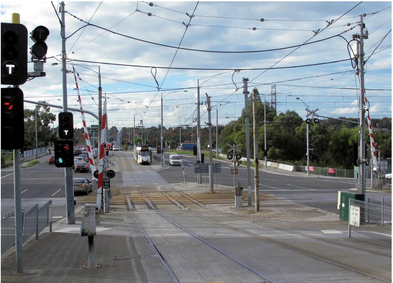
*Tramway level crossing at Burke Road Gardiner on 19 April 2012, looking north. A Z3 class tram is waiting at the traffic lights before proceeding to the city, while the tramway 'T' traffic lights that replaced the original disc signals are prominent on the left. Note the catch point in the foreground. This scene is now disappearing under the works of the level crossing replacement project. Photograph by Mal Rowe.*
