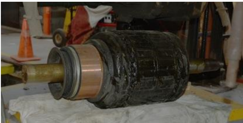
An armature at Ballarat Tramways showing the commutator. Photo: Mal Rowe
