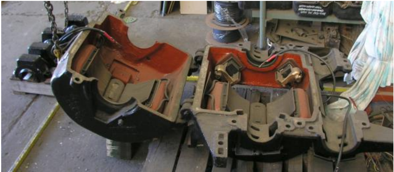
An early tram motor 'cracked open' at Bendigo Tramways showing the field coils and brush holders. Photo: Mal Rowe
